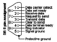
Do not use the #4 DTR (Data Terminal Ready) pin for single port PTT control despite what the AGWPE Help file or AGWPE web site may say. The DTR pin is used by AGWPE only if you <u>interface a second radio</u> and use AGWPE's <u>Dual Port</u> feature to control PTT on a radio attached to AGWPE port #2. DTR will not be triggered if AGWPE is set to use only a single port/radio.
