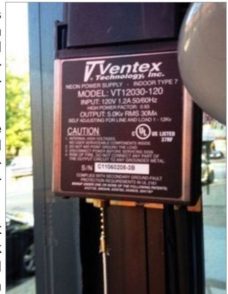
This Ventex Technology neon sign power supply was found to be a strong source of radio interference in the affected neighborhood of Evanston. [Kermit Carlson, W9XA, photo]
