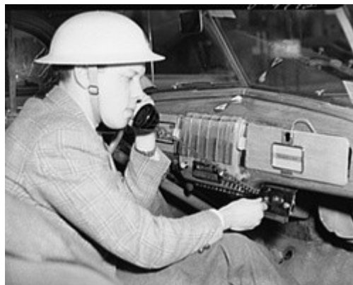
WERS licenses were given to communities and not individuals, but participants had to hold an Amateur Radio license. Civil Defense radio volunteers transformed the auto radio in this auxiliary police car into a short-wave War Emergency Radio Service set, permitting auxiliary police communications officers to maintain two-way contact with their control center. [Farm Security Administration/Office of War Information photo]
