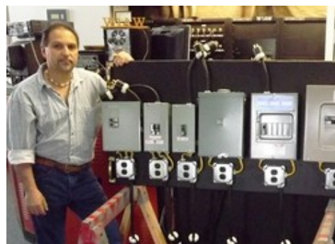
W1AW Station Manager Joe Carcia, NJ1Q, with the AFCI test stand. [Mike Gruber, W1MG, photo]
