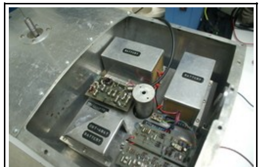
The inner workings of the newly functional OSCAR I satellite at ARRL Headquarters. This bird will be on display at the ARRL EXPO at the Dayton Hamvention, transmitting "HI HI," just as it did from space 50 years ago. See a larger photo here . [S. Khrystyne Keane, K1SFA, Photo]
