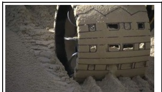
The tires on the new Mars rover -- set to launch in November or December 2011 -- will display the letters JPL in Morse code. [Photo courtesy of NASA/JPL]
