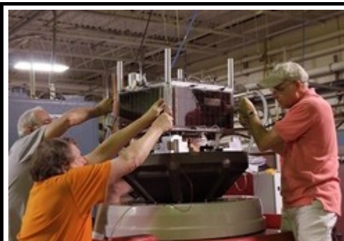
ARISSat-1 team members prepare the nano-satellite for vibration testing at the Johnson Space Center in Houston, Texas. [Dave Jordan, AA4KN, Photo]
