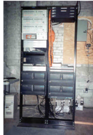
The digital system that was used to record inputs from all the cameras
